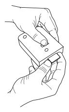
(1) Push nib up on the back of the nightlatch. Whilst holding the nib up pull out the latch.
